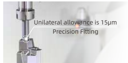
04-Verification of Position Compensation Accuracy
